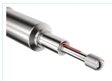
The option VH should to be chosen, if the sensor is used in liquids (oil, water, ...) or if fast pressure variations may occur. By milling plane surfaces on parts of the mechanics (see picture red marked) the pressure balance or venting of the inside area will be improved.
