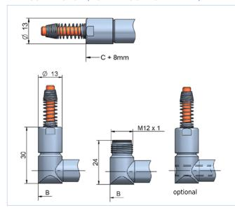
Sensors with cable output have a cable fitting and a spring for bend protection of the cable. For installation, the bending radius should not be less than 3 times the cable diameter. The standard cable length is 2 m.
