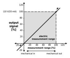
The output signal is referring to the electric measuring range. If the sensor is operated outside the measuring range or the measuring range is exceeded, the signal is also outside the defined range (i.e. > 10V/20 mA or < 0 V/4 mA, in the graph: > 100 % or < 0 %). Please keep this in mind for control systems with cable break detection lower than 4 mA or for a maximum input voltage > 10 V of measuring instruments. If necessary install the sensor **before** connecting to the PLC.
